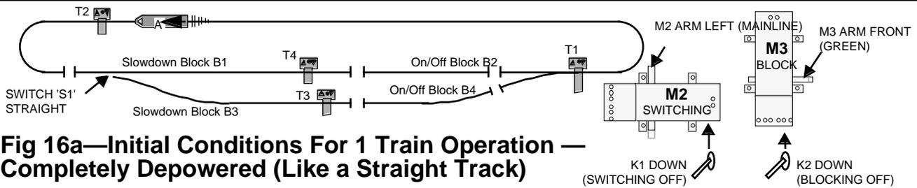
**Fig 16a—Initial Conditions For 1 Train Operation — Completely Depowered (Like a Straight Track)**
