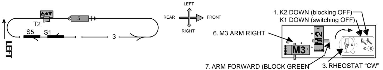
**Fig 43a Initial Conditions - 1 Train—No Controls** (Single train travels on thru Track 3—controls not operating)
