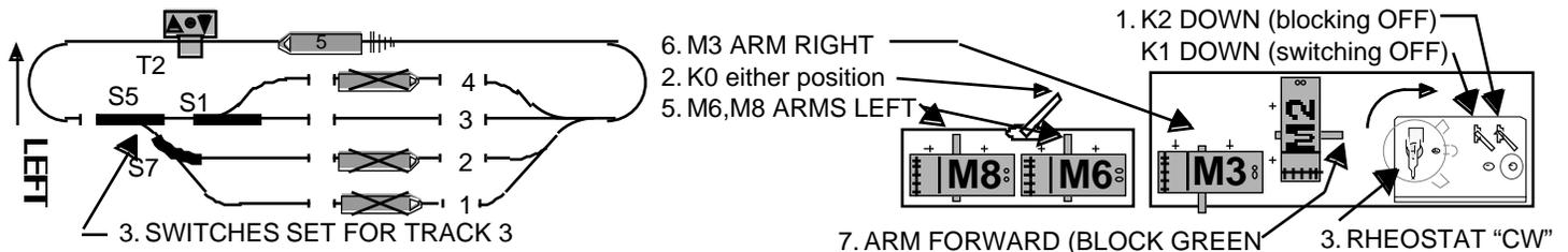
**Fig 44a Initial Conditions - 1 Train—No Controls Operating** (Single train travels on Track 3)
