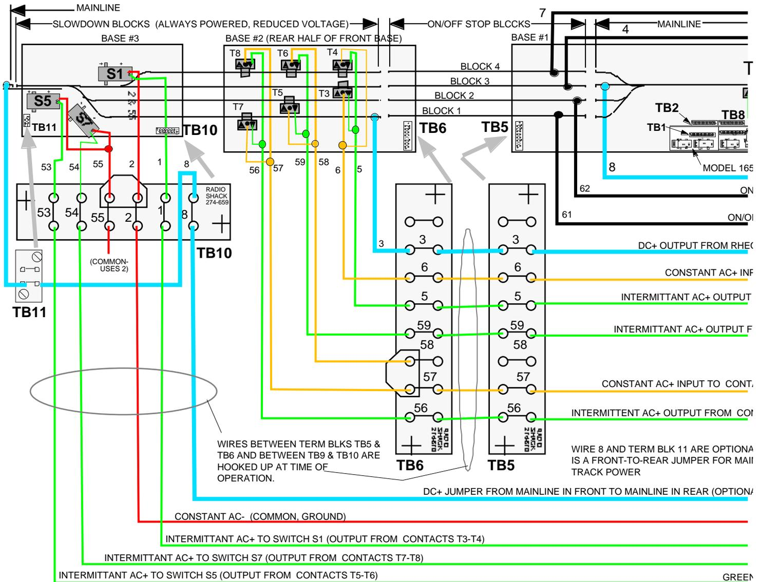
**Summary:** Use this wiring sheet **ONLY** if you are building the front track unit in 2 pieces—that is, Base #1 and Base #2 are separate pieces.
