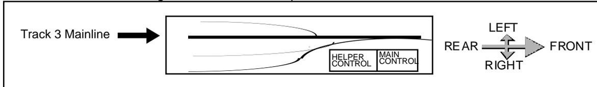
This section guides you thru wiring the mainline track (Track 3) first, using only the Main Control. Later you wire track 4. Still later you wire Tracks 1 and 2 and the Helper Control.
