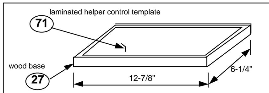
Figure 72 Wood Base With Laminated Template Attached
