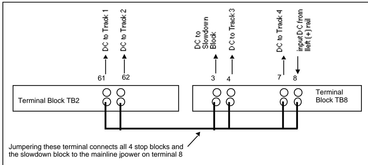
Figure 75 Jumpering Tracks To Operate Without Control Units
