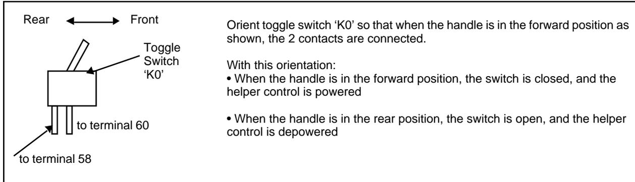
Figure 74 Orientation of Toggle Switch K0
