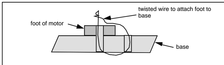
Figure 73 Using Twisted Wire to Attach Foot of Switch Motor to Wood Base
